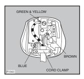
The wire coloured green and yellow must be connected to the terminal marked with the letter «E» or by the earth symbol = or coloured green and vellow.
